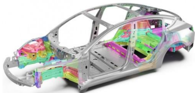
Model 3 body structure 171 pieces of metal highlighted
